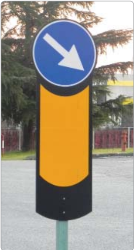
mm. 350x1200 disco Ø 400 rifr. cl.2S fig. 82 o 83 C.d.S. palo PVC mm.60x60x2000
